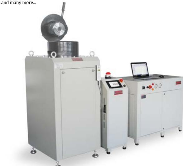
BMT-ST Shaking Table is designed to perform earthquake simulation in a workshop or lab to test earthquake effects on different products. In has a rigid base frame and a moving table that is connected with an Electro-Mechanical or hydraulic actuator controlled by BESMAK® dynamic controller and simulation software.
