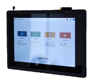
Note: Display Unit has built-in test software having same features as PC. Software.
